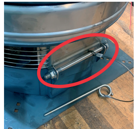
3 Remove fan head from base Using a 13mm wrench (bolt head) and 1/2" socket (nut).
