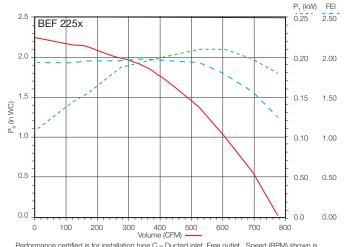
Performance certified is for installation type C – Ducted inlet, Free outlet. Speed (RPM) shown is nominal. Performance is based on actual speed of test. Performance ratings do not include the effects of appurtenances (accessories).
