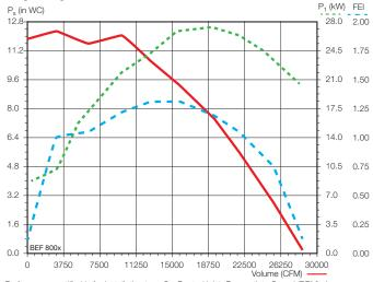
Performance certified is for installation type C – Ducted inlet, Free outlet. Speed (RPM) shown is nominal. Performance is based on actual speed of test. Performance ratings do not include the effects of appurtenances (accessories).
