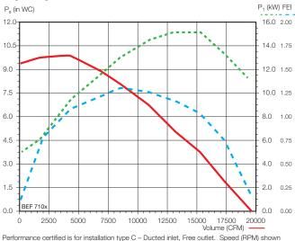
Performance certified is for installation type C – Ducted inlet, Free outlet. Speed (HPM) snown is nominal. Performance is based on actual speed of test. Performance ratings do not include the effects of appurtenances (accessories).
