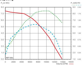
Performance certified is for installation type C – Ducted inlet, Free outlet. Speed (RPM) shown is nominal. Performance is based on actual speed of test. Performance ratings do not include the effects of appurtenances (accessories).
