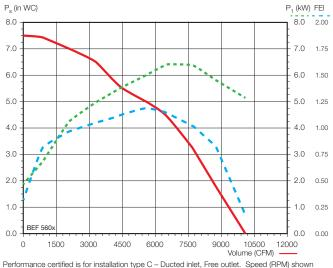
Performance certified is for installation type C – Ducted Inlet, Free outlet. Speed (HFM) shown is nominal. Performance is based on actual speed of test. Performance ratings do not include the effects of appurtenances (accessories).
