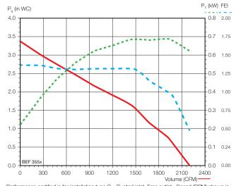
Performance certified is for installation type C – Ducted inlet, Free outlet. Speed (RPM) shown is nominal. Performance is based on actual speed of test. Performance ratings do not include the effects of appurtenances (accessories).
