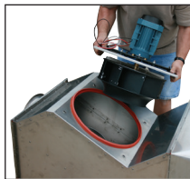
Removal of drive unit
