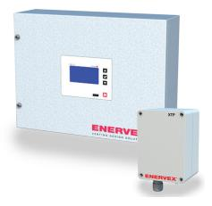
The EBC31 can be configured either by using the LCD dot display and buttons, or by using the integrated webserver, which also allows remote monitoring and firmware upgrades. Two RS485 ports can be used for and BACnet communication, and one expansion board can be used for future hardware upgrades.
