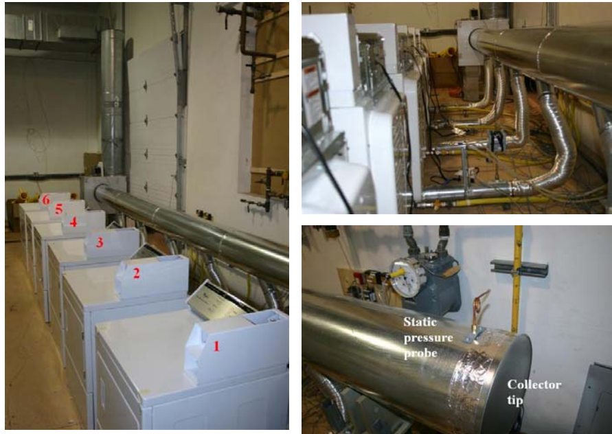
Figure 11: Multiple dryer test bench in NGTC's laboratory
