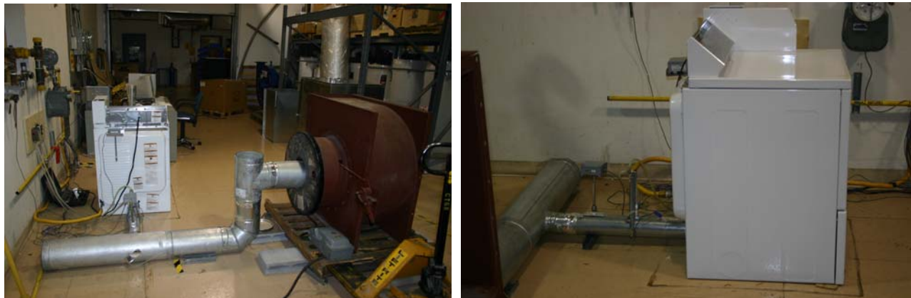
Figure 8: Set-up to study the effect of fan-assisted evacuation on dryer performance
