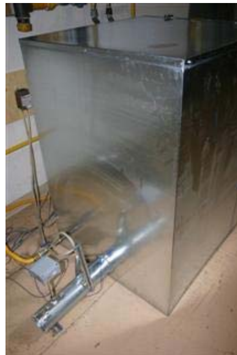
Figure 7: Dryer air-tight metal casing
