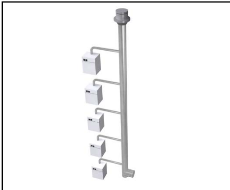
Fig. 4: Common shaft with constant speed exhaust system
