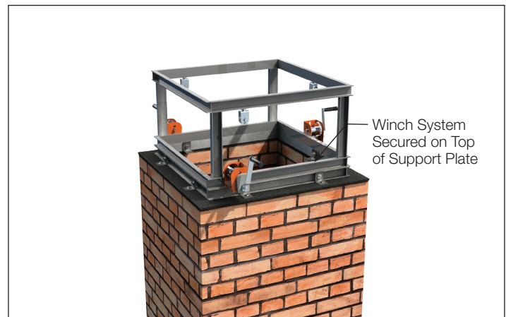
Fig 12-6: Winch System Installed
