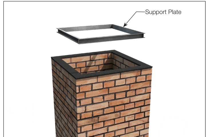
Fig 12-2: Support Frame Installation
