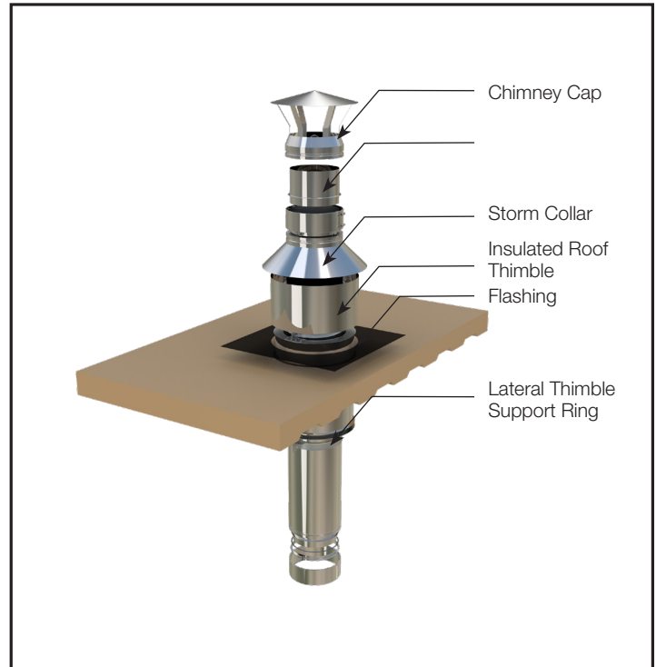
Fig 8-1: Roof Assembly Details
