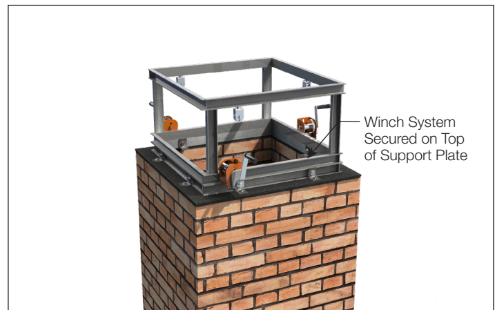
Fig 12-6: Winch System Installed
